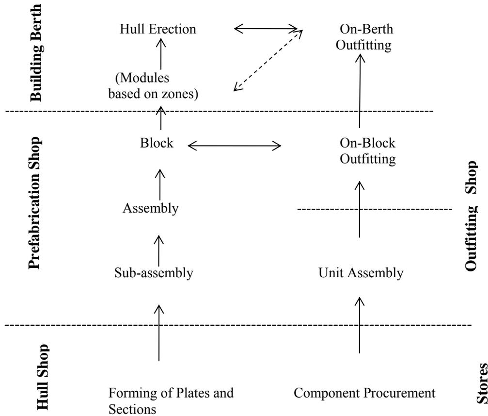
**Fig.3 Modern Ship Production Levels**
