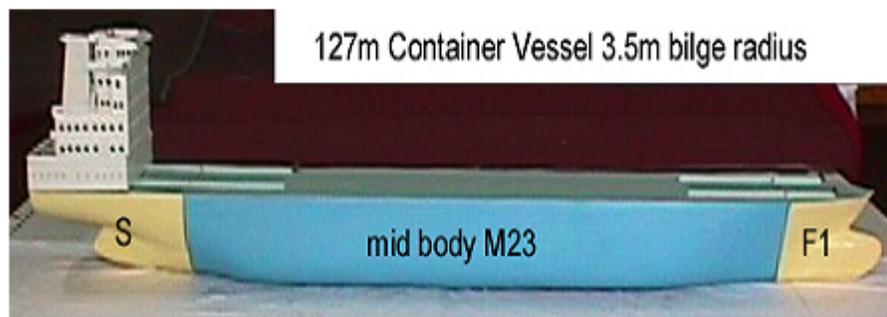
**Fig. 6. Three of the 12 ship forms generated out of the hull modules**
