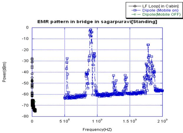
Figure 2: EMR Pattern in Bridge of Research vessel-1(Standing)
