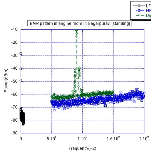
Figure 5 : EMR Pattern in Engine room in Research Vessel-1 (Standing) near transformer
