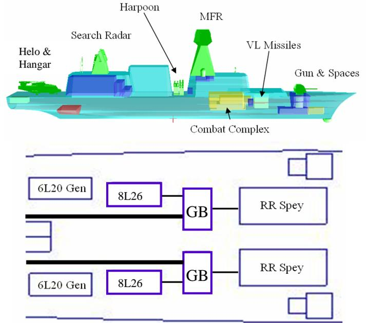
Fig. 4. Details of the CODOG vessel.
