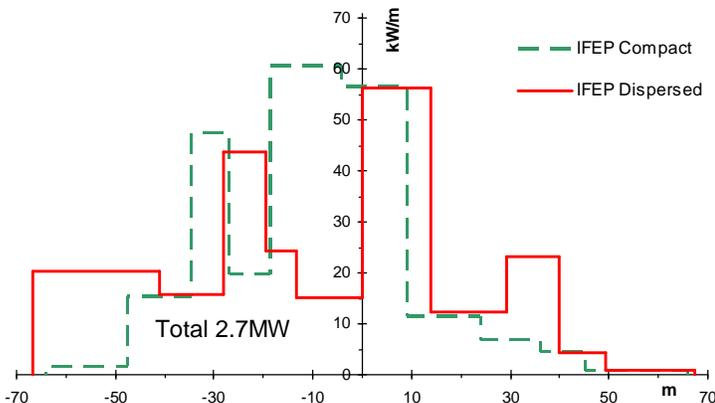
Fig. 13. IFEP-dispersed variant waste radiant heat longitudinal distribution.
