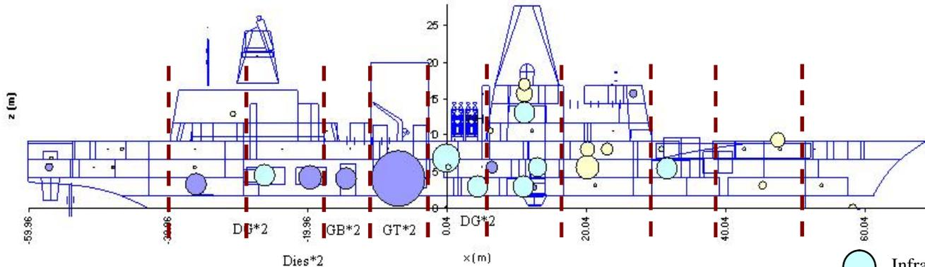
Fig. 5. CODOG (baseline) waste radiant heat
