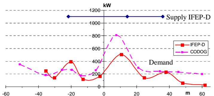
Fig. 14. Comparison of chilled water demands for CODOG and IFEP-dispersed variants.
