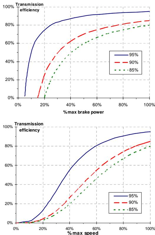
Fig. 1. Required part load efficiencies to maintain a constant transmission loss for full power transmission efficiencies of 95, 90 and 85%
