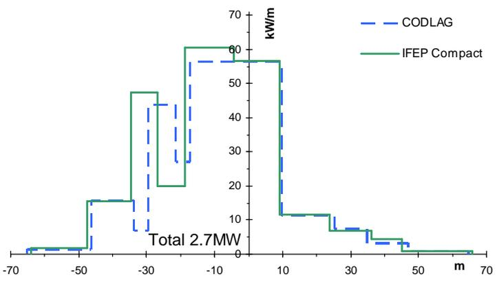
Fig. 11. IFEP-compact variant waste radiant heat longitudinal distribution.
