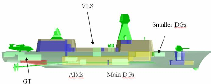
Fig. 12. Dispersed IFEP variant machinery locations.
