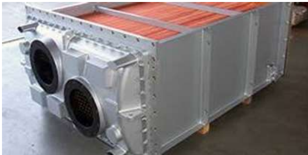
A New Air Cooler - Air Side is Red Coloured (Fins) Air Flows Top to Bottom Flanges on the Left are for Cooling Water (Tubes) Cooling Water Flows from the lower right SW inlet to the upper left SW outlet in this cooler
