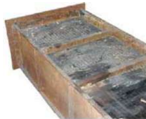
Cassette type charge air cooler received at our workshops
