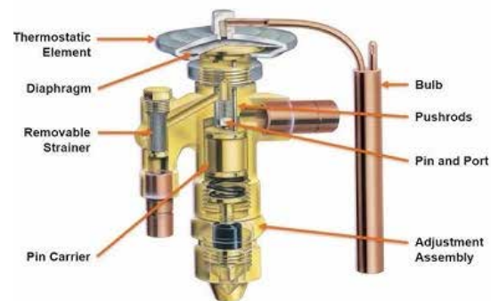
Parts of a Thermostatic Expansion Valve
