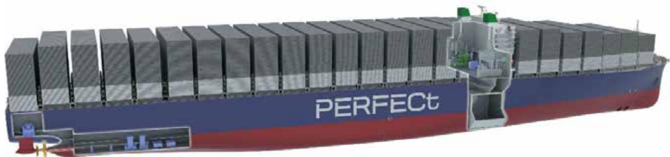
Figure 3. Computer model of the proposed LNG COGES-powered 20,000 TEU vessel, by DNV Group.
