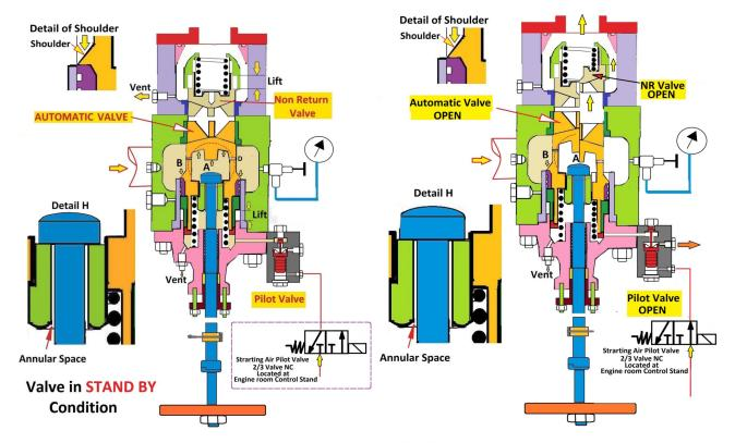
Starting Air pressure acting upon the upper side of the Automatic starting Stop Valve + the Spring force is GREATER THAN the Starting Air pressure acting upon the shoulder and hence remains CLOSED
