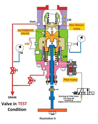
When a movement is ordered from the Bridge, the telegraph is answered and the Starting Lever is shifted to "START" position. The starting lever mechanically
