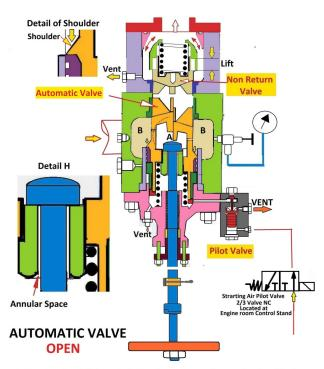
As the chamber "A" is vented, the air pressure acting on the shoulder is greater than the spring force and opens the automatic valve against the spring force. This sequence is shown on the right half of the illustration
