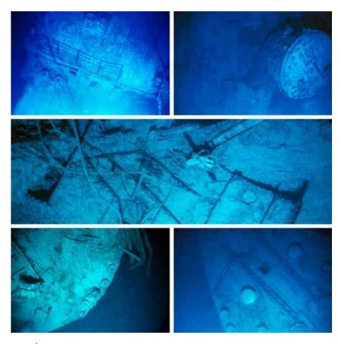
but the stern is ruined from damage during the sinking, mostly because of her almost vertical dive into the depths of the North Atlantic, after shearing off from the forward section.
