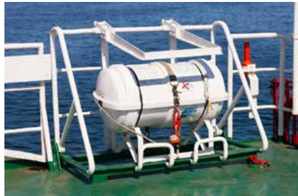
A Life Raft shown with a Hydrostatic Release Unit
