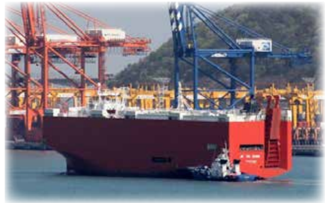
Arrangements Astern on the "Nosac Taishan" with the Stern Ramp Raised. Note the Position of the Bridge Forward
