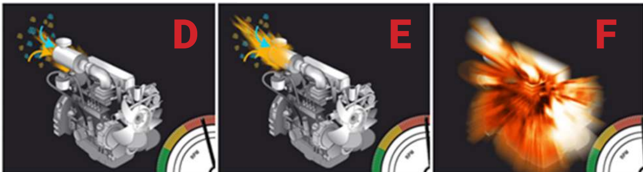
Engine races at RPM above it's limit, exh. and inlet valves will be unable to seat efficiently
