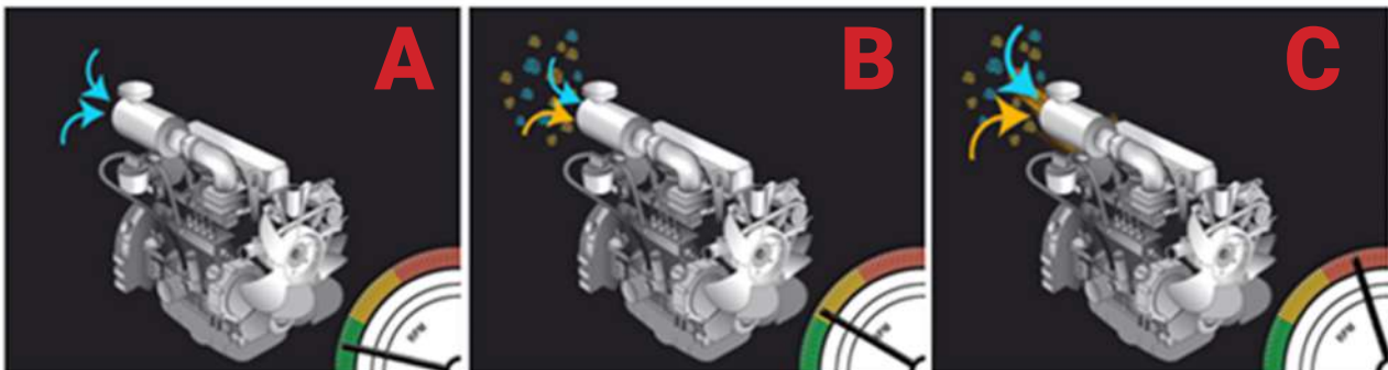
Dual Fuel Running - Consumed Gas adds energy causing diesel fuel to reduce
