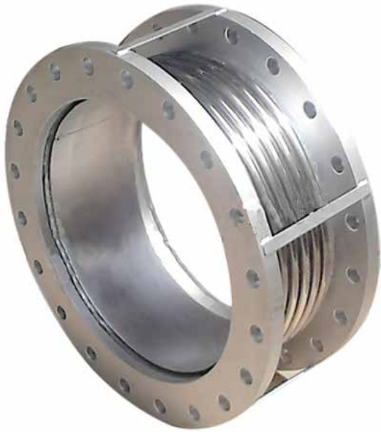
Image Courtesy indiamart // Note the stainless steel sleeve in the interior and the corrugated bellows on the outside. // The free, unwelded end of the sleeve is clearly visible, which allows for longitudinal expansion. // This stainless steel sleeve is free at one end (gas outlet end) and welded to the flange at the other end (gas inlet end) // Note both flanges are the same size, same number of bolt holes, so they can be fitted either way. // Note the flat strips welded to each flange.
