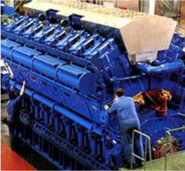
Courtesy dieselduck.net // A 16 cylinder V type Engine (Image 1) Image 1 as referred to in text
