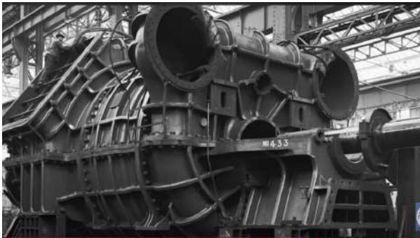
The 410 ton Low Pressure Turbine - although built for Hull 433, it was the same as the Titanic (Hull 401), developing 16000 shaft horse power. Though built for Hull No. 433, the same design of turbine was used in Hull No. 401, the Titanic.
