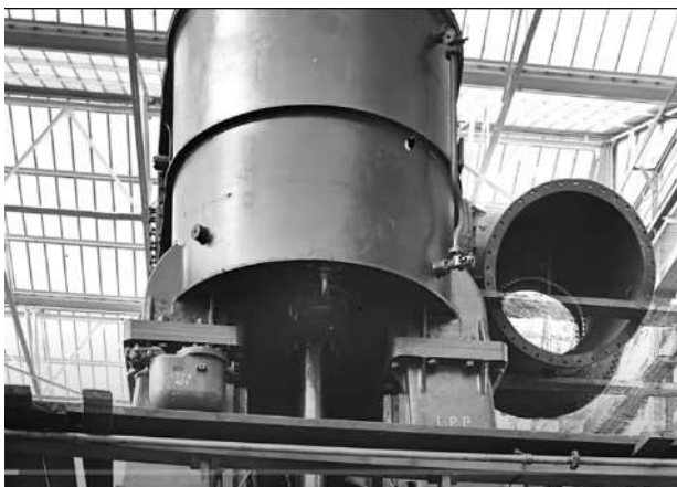
Triple Expansion Engine - Upper Portion showing the LP Unit
