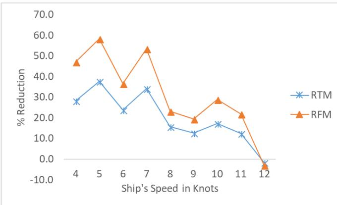
**Figure 6 Comparison of Percentage Reduction in Total resistance and frictional resistance of ship for Injection rate of 1.0 CFM**
