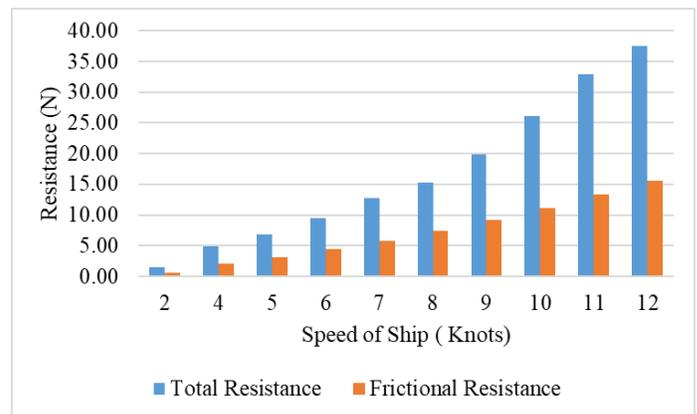
Figure 3 Towing tank results without the injection of microbubbles
