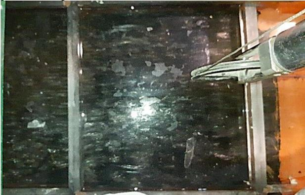
**Figure 11 Distribution of bubbles below the hull at a speed of 6 knots and air injection rate of 1.0 CFM**
