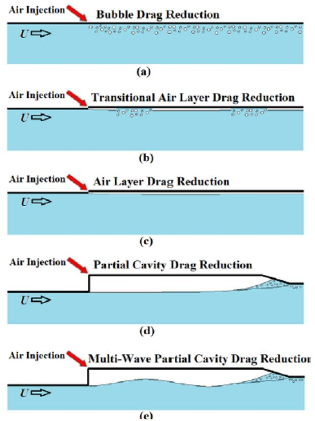
Figure 4 Different MBDR techniques used to reduce frictional drag (Mäkiharju, et al., 2012) & (Jinho, et al., 2014).
