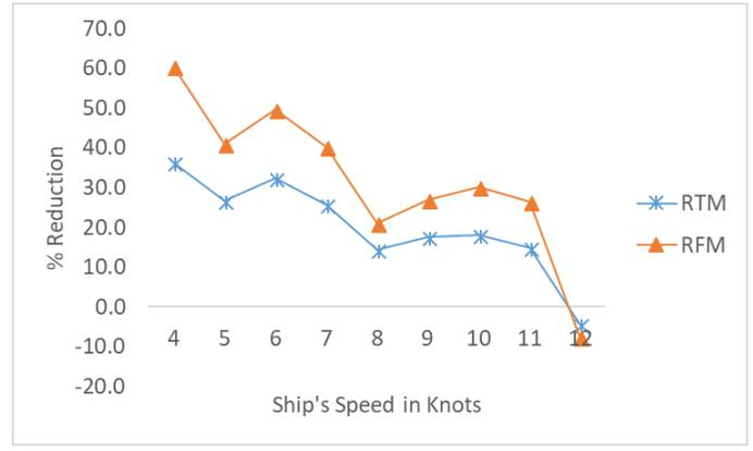
**Figure 7 Comparison of Percentage Reduction in Total resistance and frictional resistance of ship for Injection rate of 1.5 CFM**
