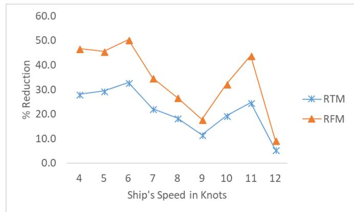
**Figure 8 Comparison of Percentage Reduction in Total resistance and frictional resistance of ship for Injection rate of 2.0 CFM**
