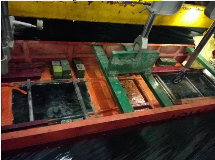
Figure 2 Acrylic sheets placed for the visualization of flow
