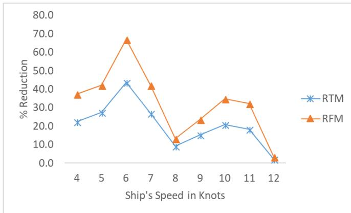
**Figure 10 Comparison of Percentage Reduction in Total resistance and frictional resistance of ship for Injection rate of 3.0 CFM**
