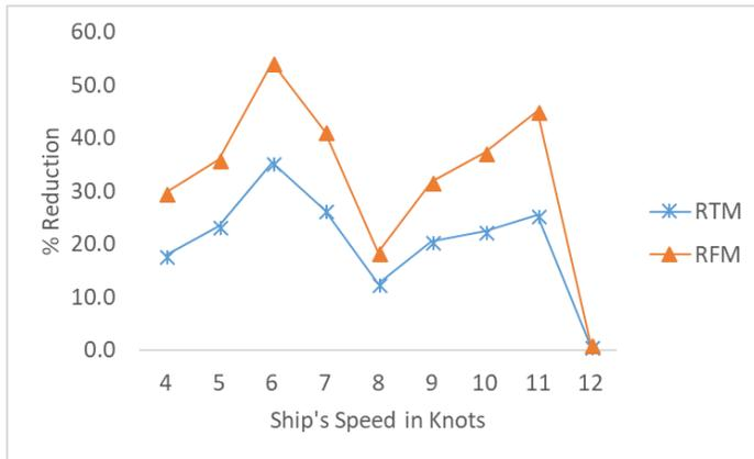
**Figure 9 Comparison of Percentage Reduction in Total resistance and frictional resistance of ship for Injection rate of 2.5 CFM**
