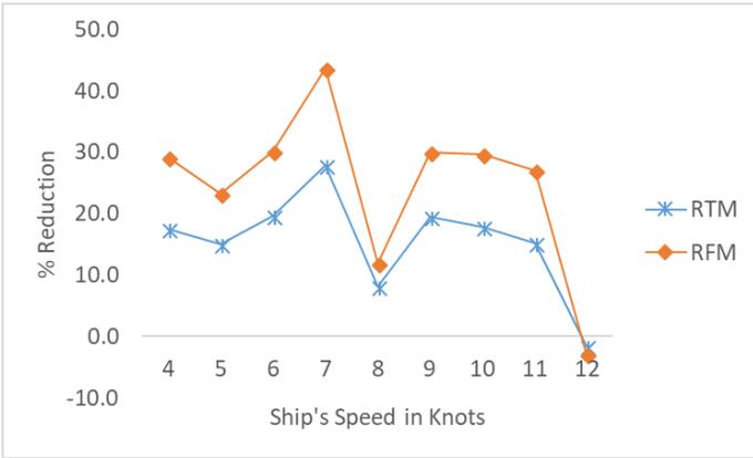
**Figure 5 Comparison of Percentage Reduction in Total resistance and frictional resistance of ship for Injection rate of 0.5 CFM**
