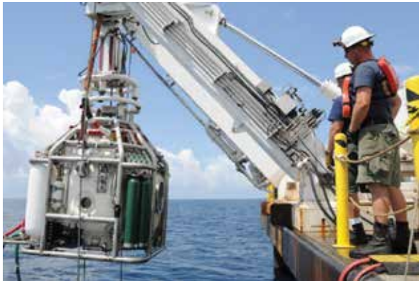
Figure.3. Diving bell launched using ship LARS
