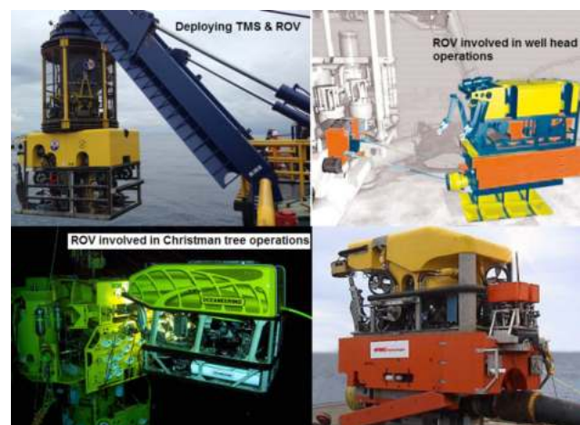
Figure.8. Work class ROVs deployed and in operation
