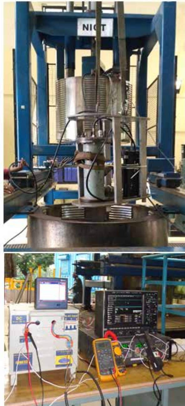
Figure. 6. View of hyperbaric testing of CB
