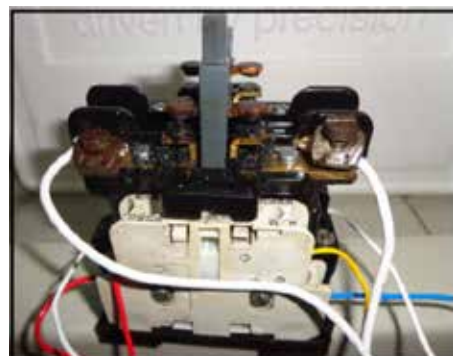
Figure. 10. Carbon particles bridging the contactor contacts
