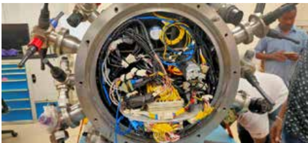
Figure. 2. 6000m depth-rated enclosure housing electronics
