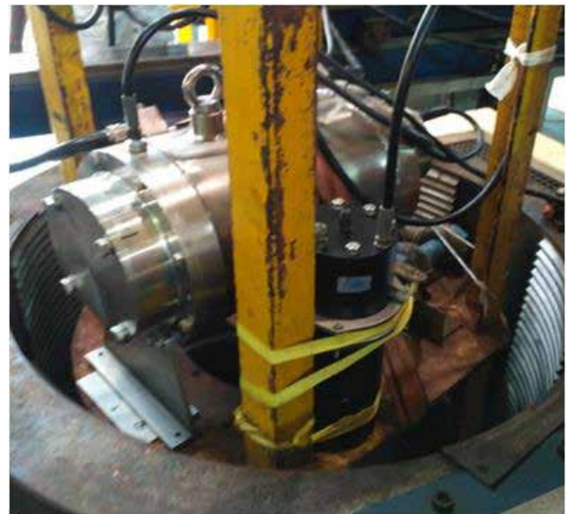
Figure. 18. Subsea motor placed in hyperbaric chamber
