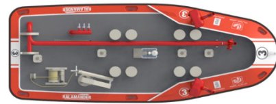
Figure 2. Aerial view of an autonomous fireboat, RALamander 2000. Adapted from [11].
