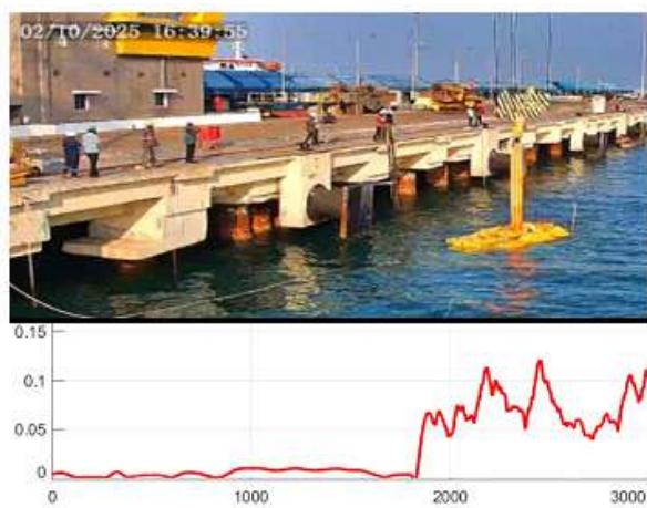
Figure.3. Identification of cut-in velocity from maneuvering test
