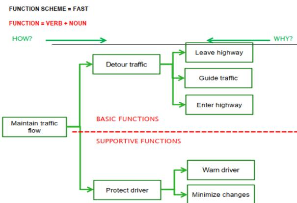
**Figure 4: FAST diagram to maintain traffic flow [16]**
