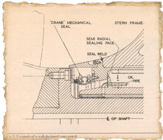
Fig 2: Example of a well-designed rope guard.
