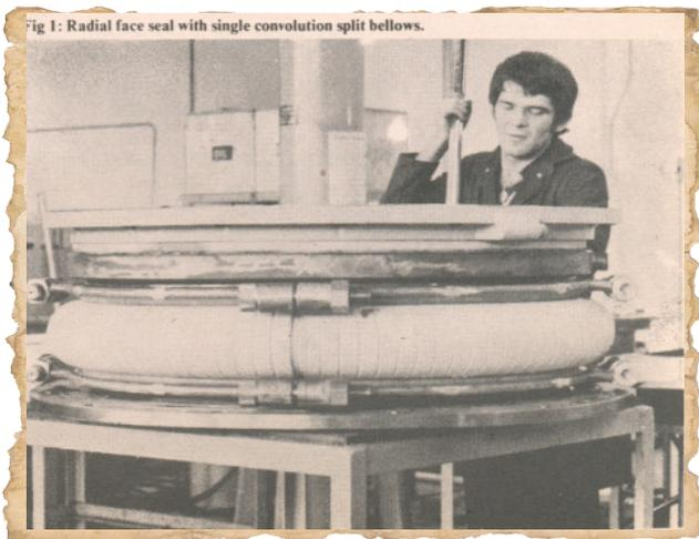
Fig 1: Radial face seal with single convolution split bellows.
