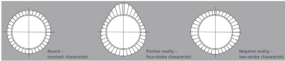
**Figure. 2: Radial pressure distribution due to ring shape (1)**
