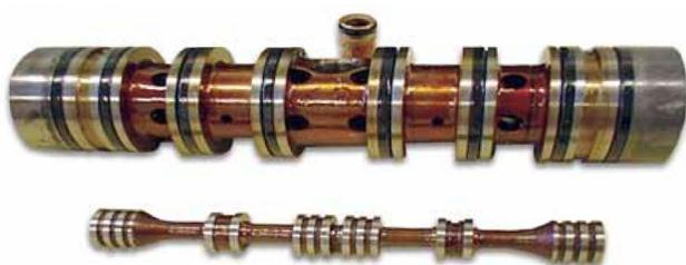
**Figure. 5: Varnish deposits on spools (Primary reason for control equipment failures.)**
