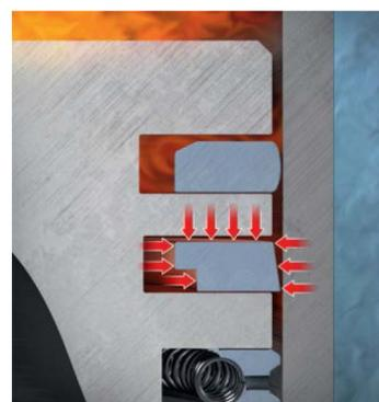
**Figure. 4: Gas pressure on a taper faced ring (2)**
