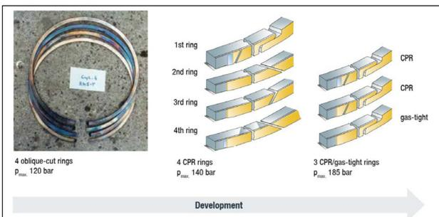
**Figure 12: 2-Stroke slow speed crosshead engine ring pack development (MAN) (5)**
