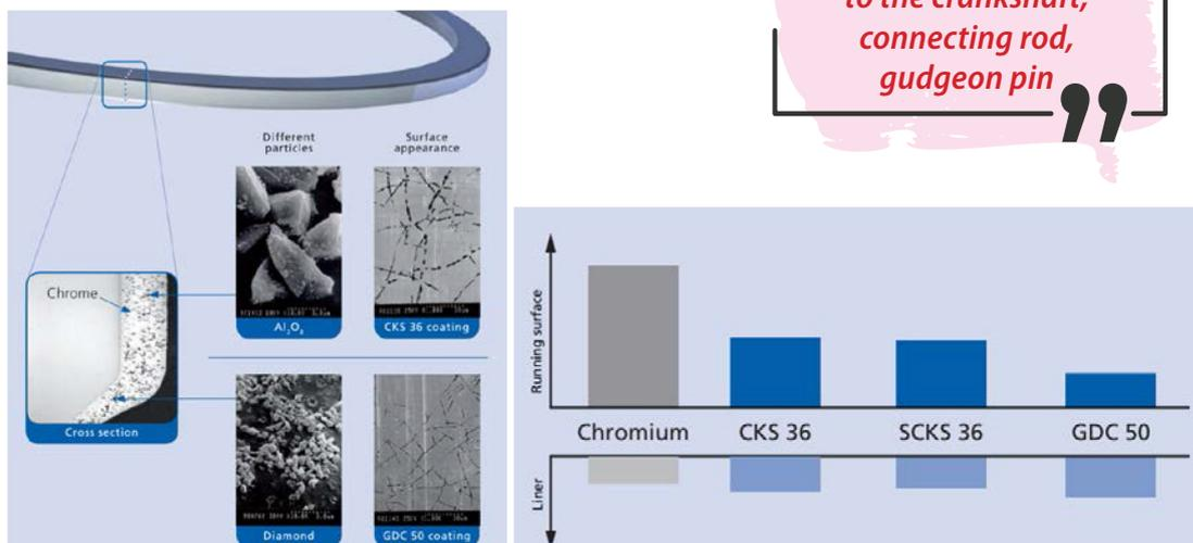
Figure 12: Chrome-ceramic (CKS), and Chrome- diamond like carbon (GDC) coating structure and running surface wear of different coatings (1)
