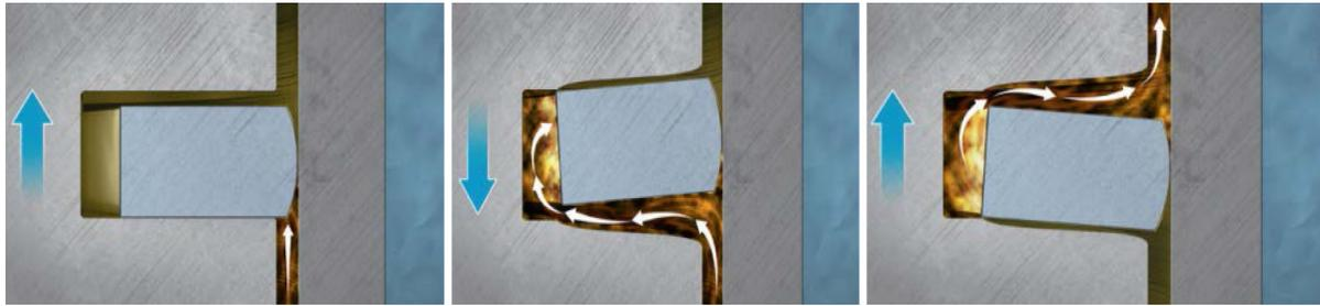
Figure. 6: (a) Sealed groove (b) leaking seal during intake (c) leaking seal during compression (2)
