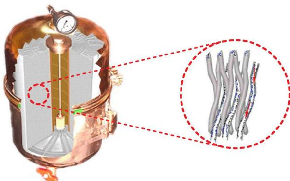
**Figure. 9: Capillary like fibres in depth filters**
