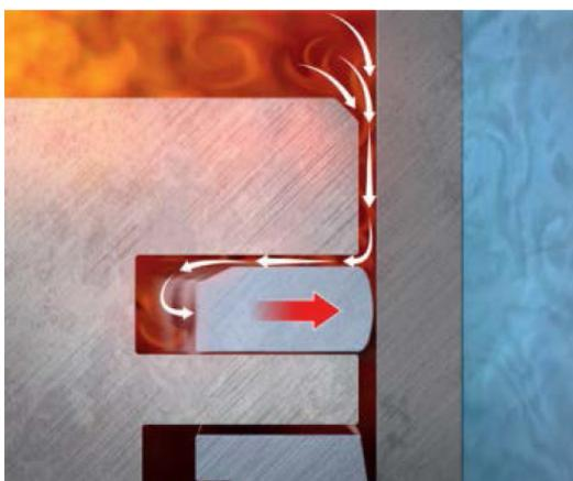
**Figure. 3: Increase in compression pressure during combustion (2)**
