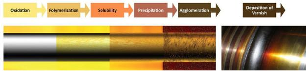
**Figure. 4: Oxidation Stages (deposits on hydraulic components)**
