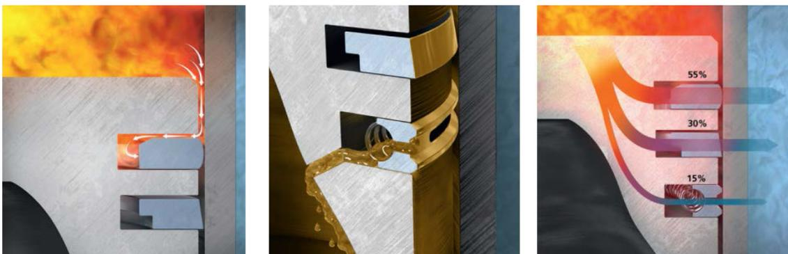
Figure. 1: Role of piston rings a) gas sealing b) oil film control c) heat dissipation (2)
