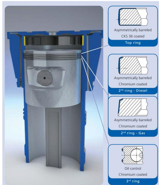
**Figure 13: Ring set for 4-Stroke TPE\*\* (1)**
