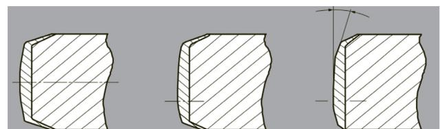
**Figure. 5: Compression ring profiles (1)**
