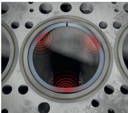
**Figure. 9: Ring flutter due to lifting of the ring from the sliding surface.**
