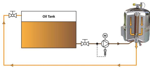
**Figure. 8: Kidney Loop filtration system with independent motor and pump**
