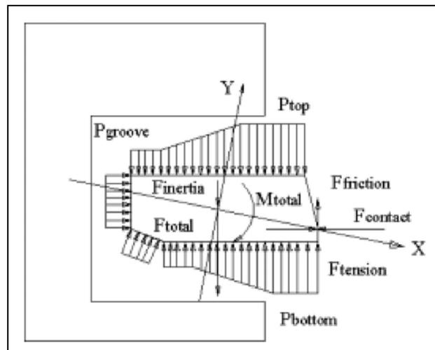
Figure. 7: Forces acting on piston ring (3)
