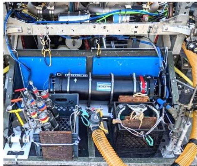
Figure 5. PMEL's hydrothermal fluid and particle sampler
