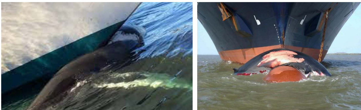
Figure 1. Images showing Dead whale struck on the Bulbous of the large ships
