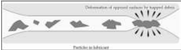
Figure 9 Contact fatigue due to entrained particles (5)
