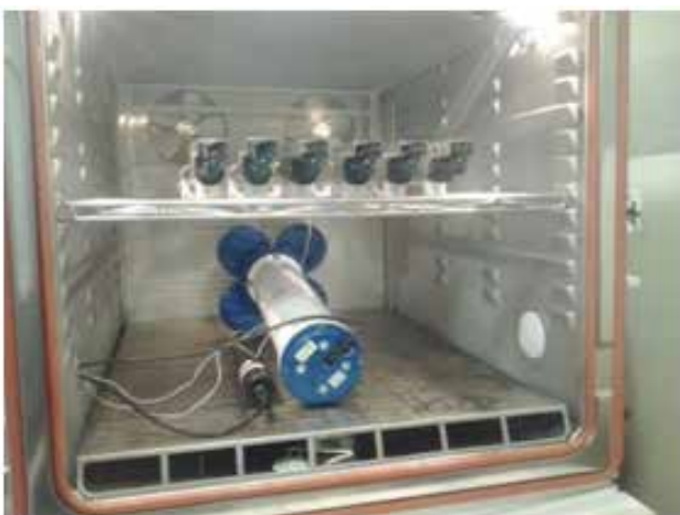
Figure.5. Qualification of sensors in environmental chamber
