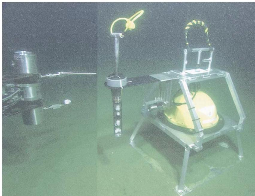
**Figure 1. Experimental apparatus on the seafloor as recorded by the video camera on ROV Ventana [1]**
