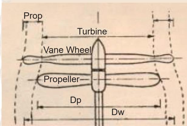
**Fig 2: Wheel and propeller wakes.**
