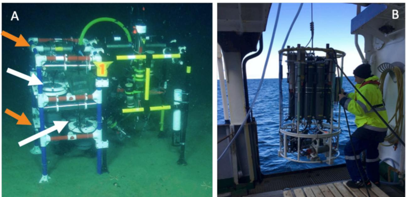
**Figure 3. Benthic lander and water sampler used in STEM- CCS experiments in North Sea [3]**
