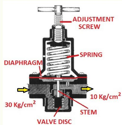
After FWE, the pressure regulator valve (97-2) was dismantled and not only was it found that the diaphragm was ruptured; the valve pin was found on the side of the valve so the same was replaced and the reversing system was restored to normal. In view of the Suez transit no further thought was given.
