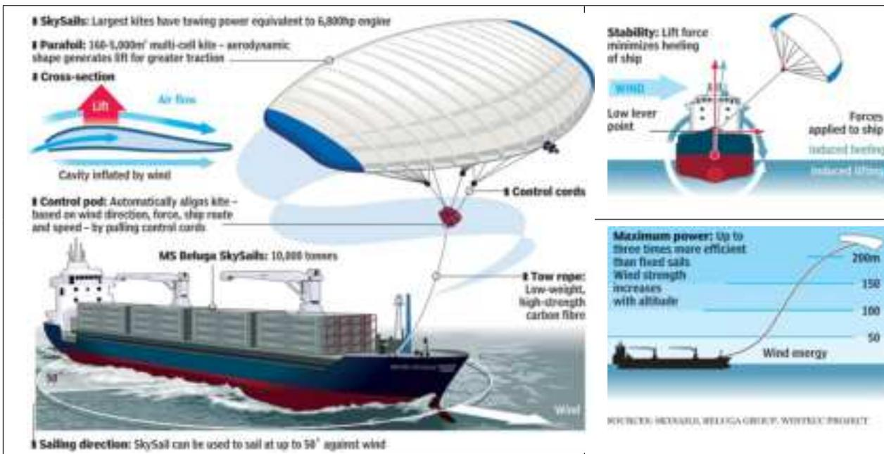
Figure. 17: MS Beluga depiction with Skysails Kite (Source: Skysails)
