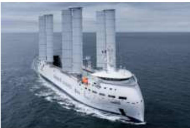
Figure. 11: Ro-Ro ship Canopée with 4x Oceanwings
