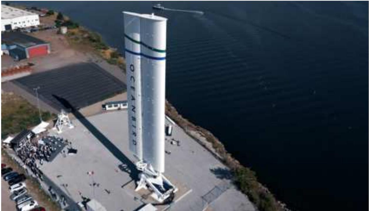
Figure. 10: Shore based prototype testing of Oceanbird Wing 560
