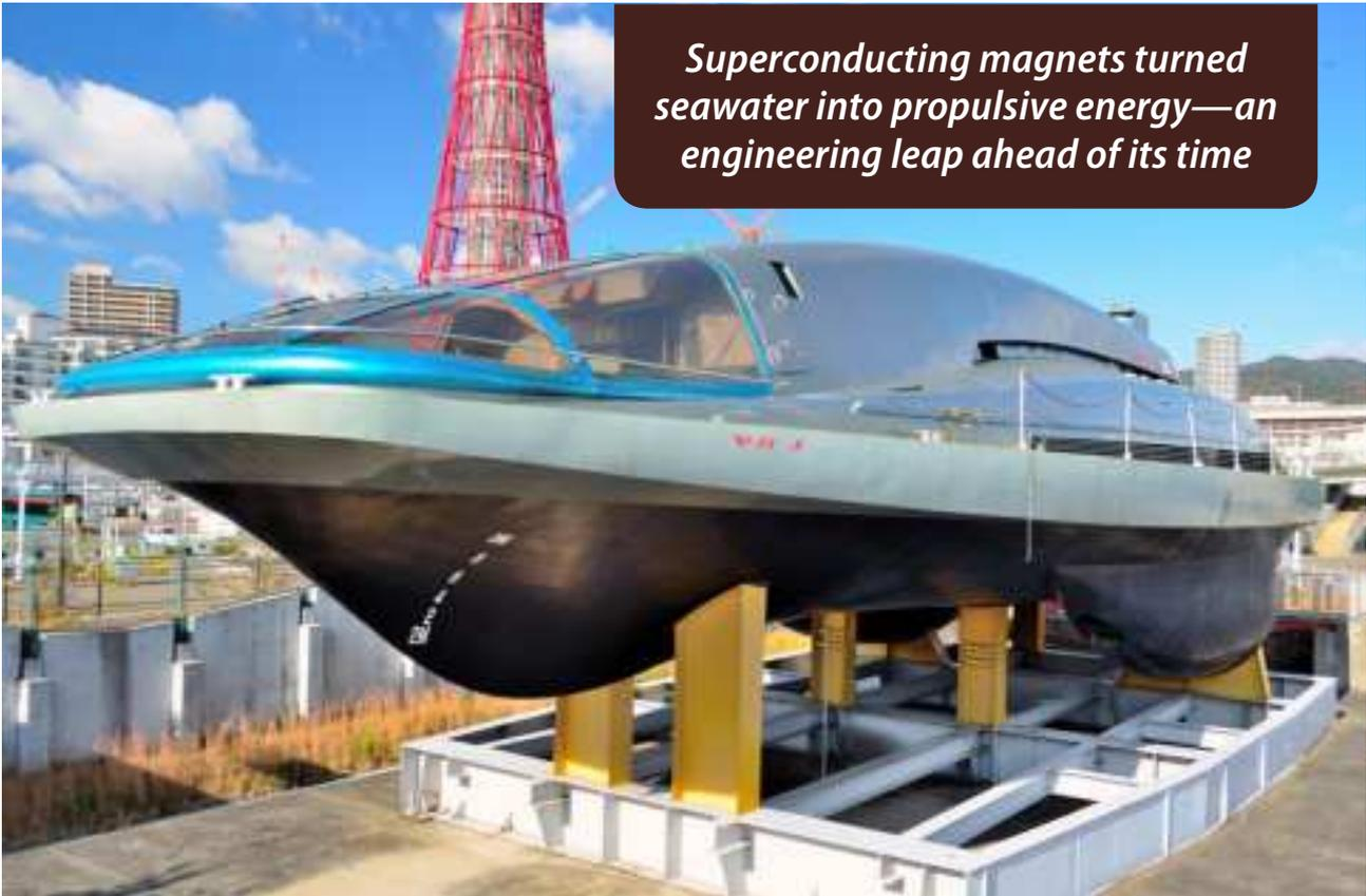
*Superconducting magnets turned seawater into propulsive energy—an engineering leap ahead of its time*
