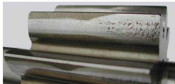
Figure 14. Pitting due to surface fatigue (5)
