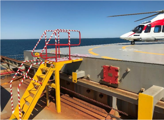
Figure 5. Helicopter hatch access requirements
