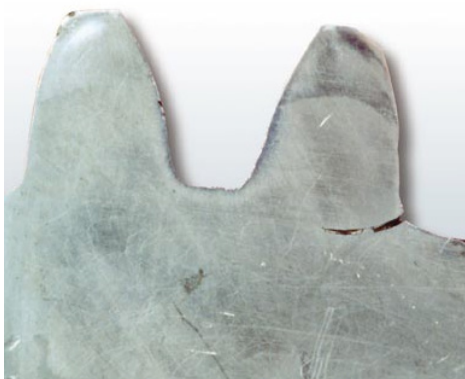
Figure 13. Bending fatigue crack at root fillet (7)
