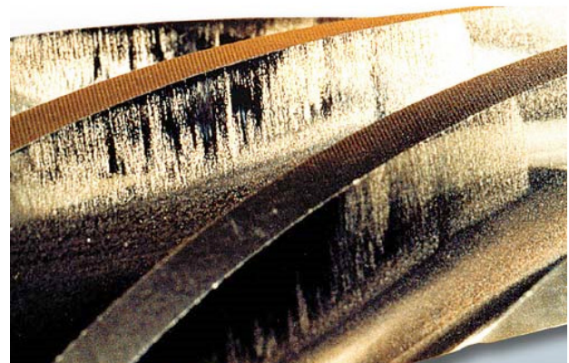
Figure 17. Destructive wear by (L) Abrasion (6), (R) Adhesive wear (scuffing) (5)
