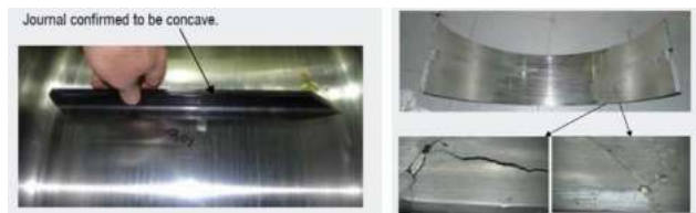
Figure 5: Main bearing failure due to concavity of pin (2)
