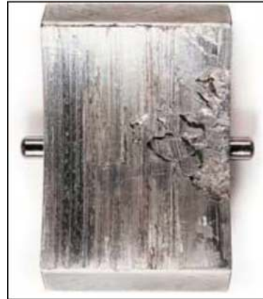
Figure 11: Flaking of bearing metal following fatigue induced cracks.
