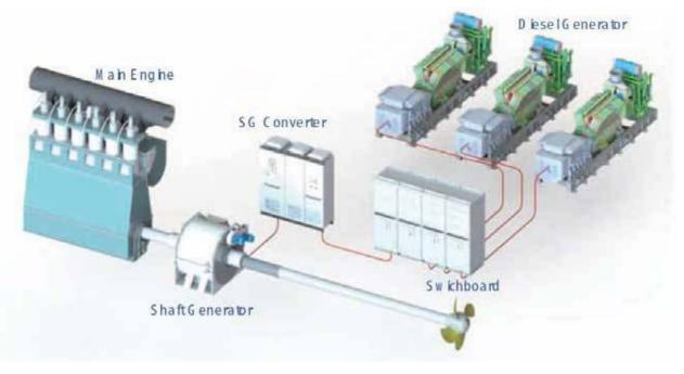
Figure 10 - LAYOUT OF SHAFT GENERATOR SYSTEM
