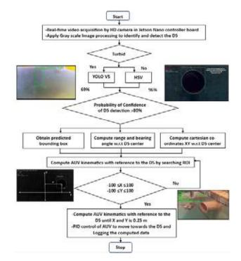
Figure 11. Decision algorithm for guidance used in VG-AUV Bearing computation
