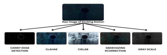
Figure 4. Different HSV techniques for dock detection
