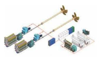
Figure 7 – Schematic layout of Medium/High speed shaft Generator (courtesy – CSSC/SMDERI)
