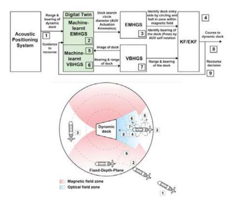
Figure 17. Concept of homing stages with the aid of DT
