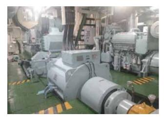
Figure 8 – Actual Picture of Medium/High Speed shaft generator (courtesy – CSSC/SMDERI)
