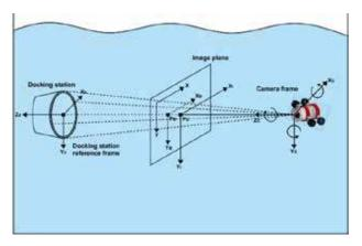
Figure 12. BI-AUV pose computation with dock in XY plane
