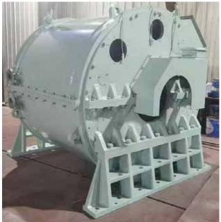
The Shaft generator is generally made to order and hence the buyers initial specification plays an important role in getting the right equipment delivered. Specification related to the range of RPM where the shaft generator is to work, and the power output VS RPM are very critical for getting maximum benefit from the Shaft Generator.
