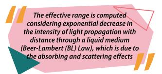
Where "*I*" is the intensity of light at a distance "*r*" from the source, "*I*<sub>0</sub>" is the initial intensity at r = 0, and " $\alpha$ " is the absorption and scattering coefficient of the water medium. A software tool based on BL law is developed using MATLAB to determine the range for the given LED light intensity, given the turbidity of sea water as the input.
