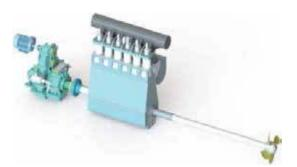
Figure 5 – Schematic layout of Gear Type Shaft Generator (courtesy – CSSC/SMDERI)
