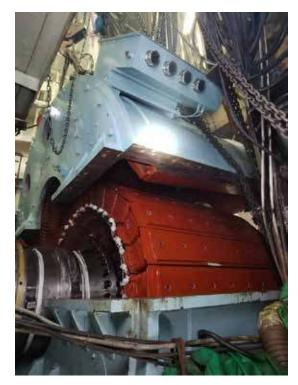
Figure 2 – Rotor and stator of Shaft generator (courtesy – CSSC/SMDERI)
