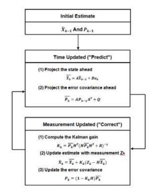
Figure 15. Principle of KF Algorithm
