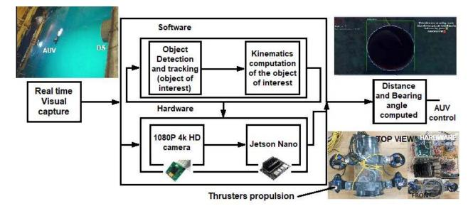
Figure 3. Image processing hardware architecture for VG
