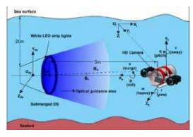
Figure 1. Concept of vision-based homing guidance
