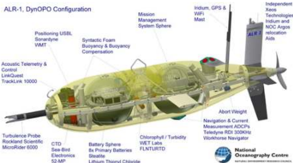
Figure. 10. AUV equipped with a subsea GPS receiver
