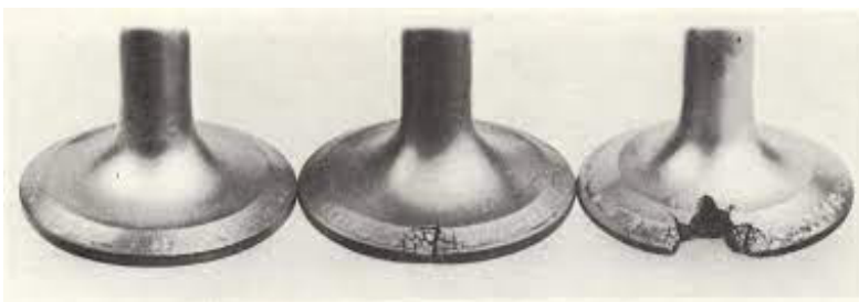
Figure. 9: Hot Corrosion of diesel engine valve (9)
