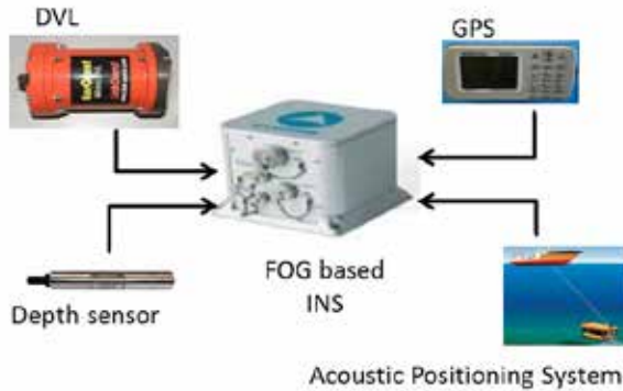
Figure.4. Architecture of aided- inertial navigation system
