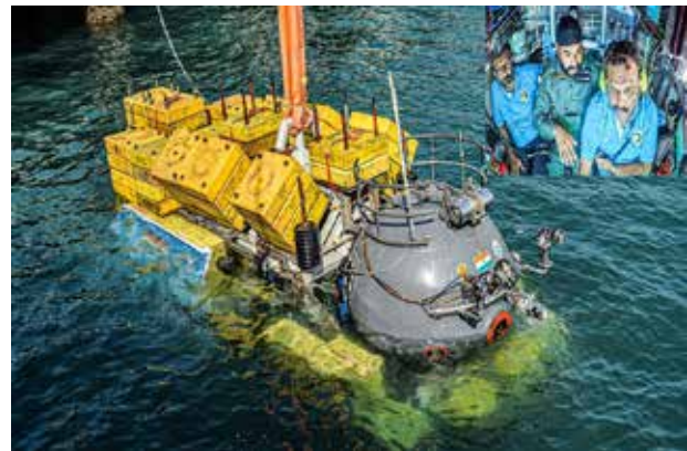
Figure.7. Matsya6000 undergoing qualification test in harbor
