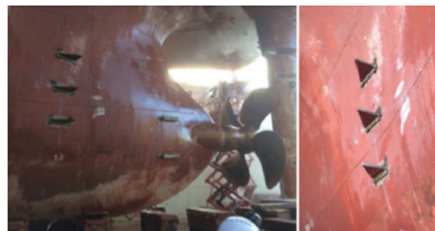
Figure. 14 Vortex generators fitted upstream of a propeller
