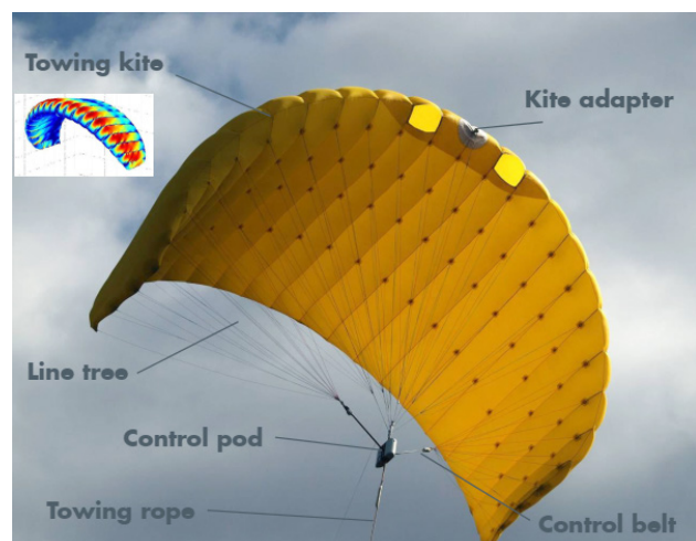
Figure. 3: Kite designed for ship propulsion
