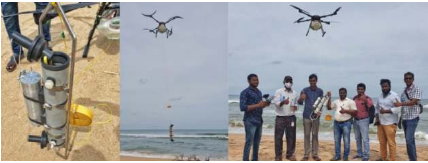
Figure 16. Automatic Sea water sample collection using Drone
