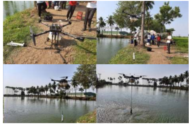
Figure 15. Sequence of operations performed with CTD data collection using Drone
