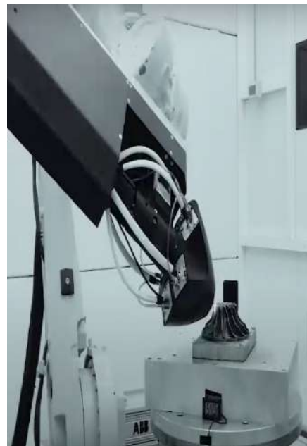
Figure.4: a) Advanced robotic arm time for 3D operation b) Robotic arm 3Dprinting impeller
