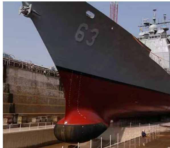
Figure. 11. View of ship hull placed sonar
