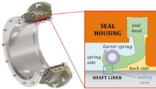
Figure 3: Stern tube seal Aft package (1)
