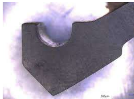
Figure. 2: Stern tube seal cross-section (1)
