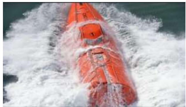
Figure 2 Slamming effect of free-fall lifeboat
