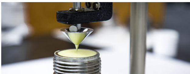
Figure 4. Cone penetration test (4)
