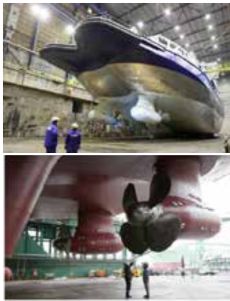
Figure.11. Podded azimuth thrusters in ice-breaking ships
