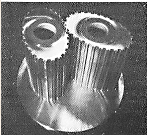
Fig 2: The oval gear wheels. ▼
