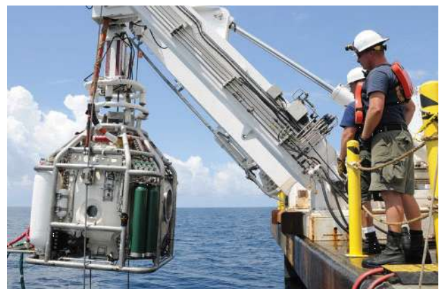
Figure 4. Diving bell launched using ship LARS
