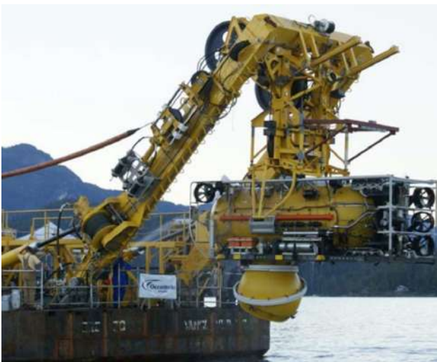
Figure 9. DSRV with hatch mating system
