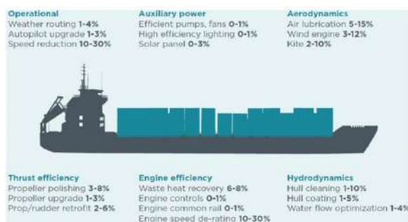
Figure 1: Potential fuel use and CO 2 reductions from various efficiency approaches for ships
