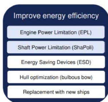
Figure 2: EEXI improvement measures if attained EEXI \geq required EEXI
