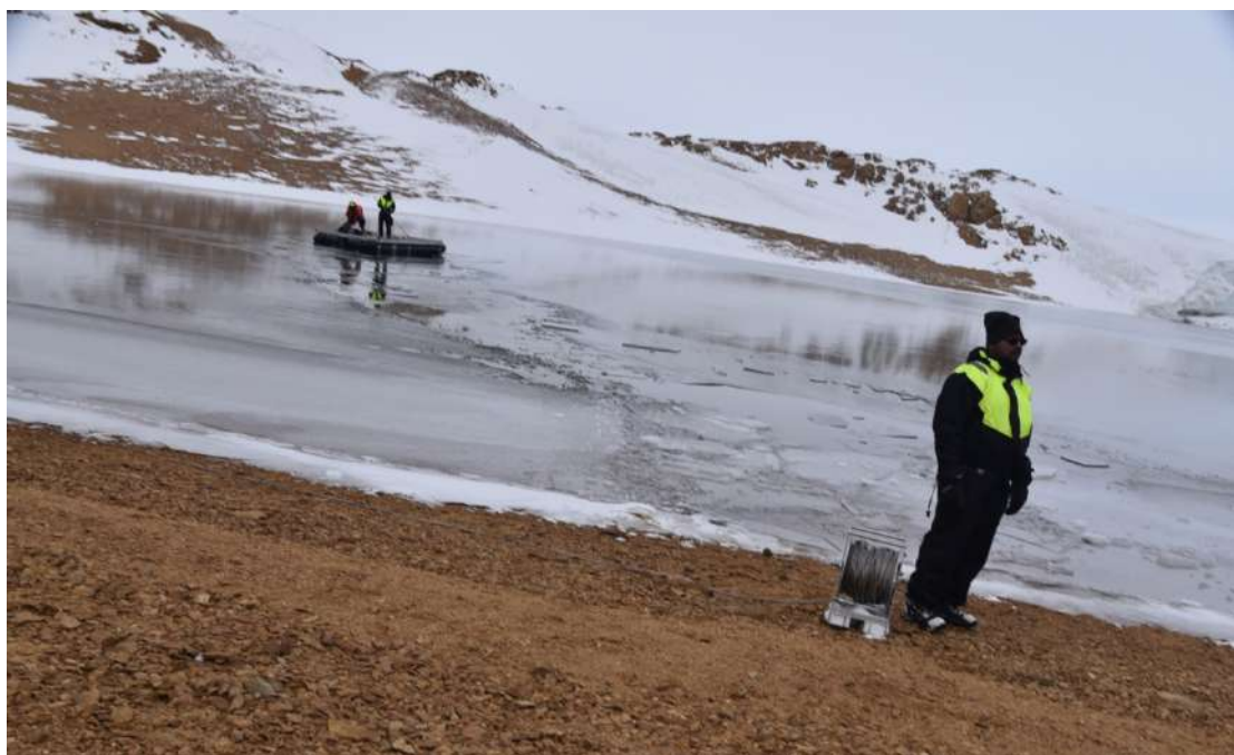
Sample collection in a deep water later with the help of a floating platform
