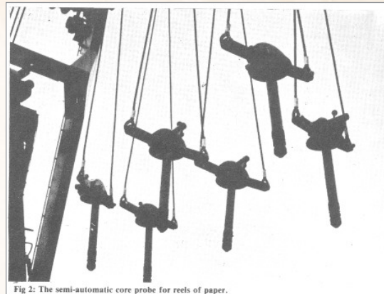
Fig 2: The semi-automatic core probe for reels of paper.
