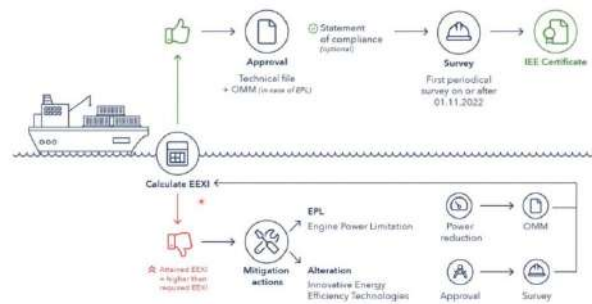
Figure 3: Procedure for issuing a certificate of conformity
