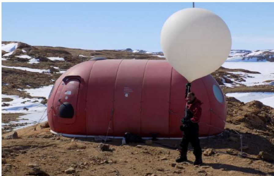
Ozonesonde is being launched at Bharati
