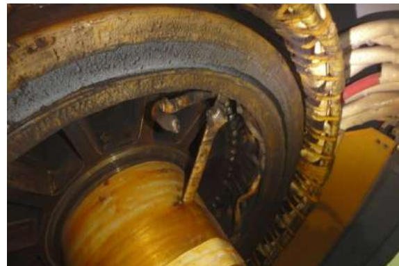
Figure 3. Rotary Diodes and Break in Main Field Winding
