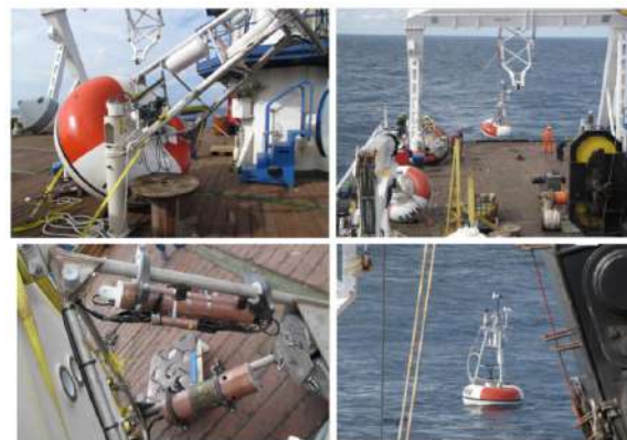
Figure.2. RAMA-BoBOA buoy deployed from NIOT Sagar Nidhi vessel in 2013
