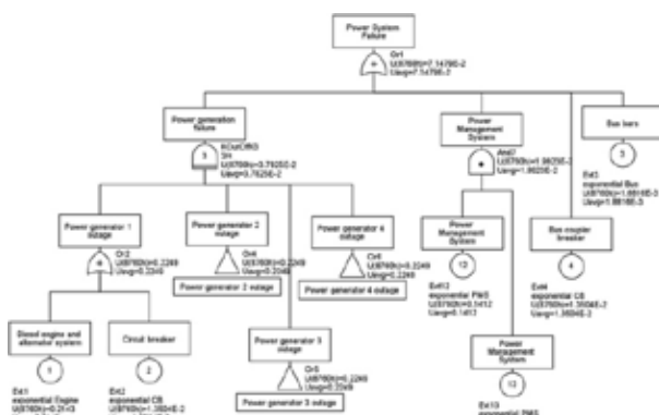
Figure 6. FTA for identifying the PoF for 3oo4 configuration
