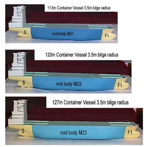
Fig. 6. Three of the 12 ship forms generated out of the hull modules
