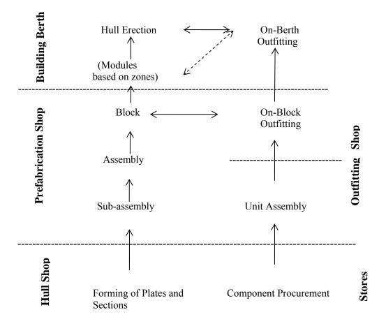
**Fig.3 Modern Ship Production Levels**
