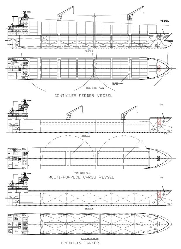
Fig. 7. Conceptual General Arrangement Drawings of three types of Vessels made from the Hull Modules
