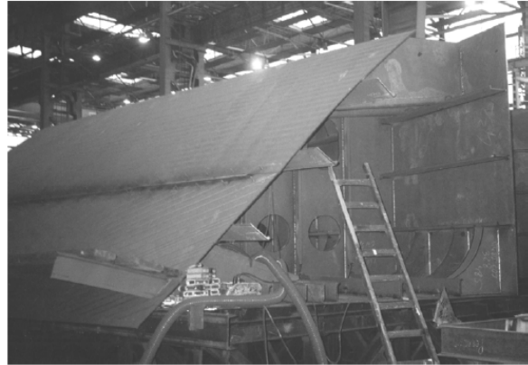
Fig. 2 Overhead manufacturing method for curved block sections
