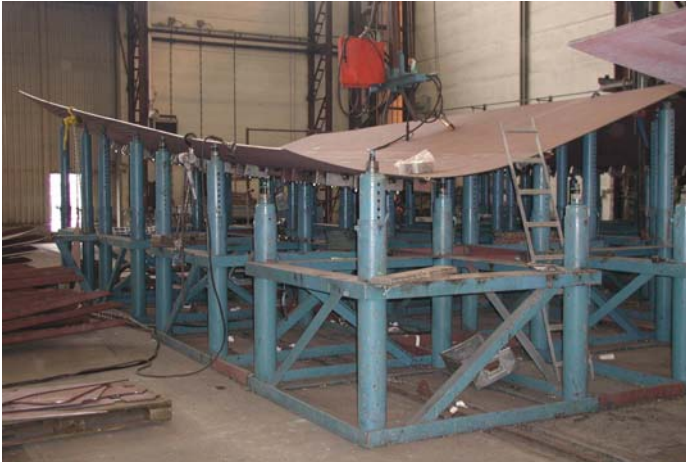
Fig. 4 Jig - pillar with applied and clamped ship hull plates
