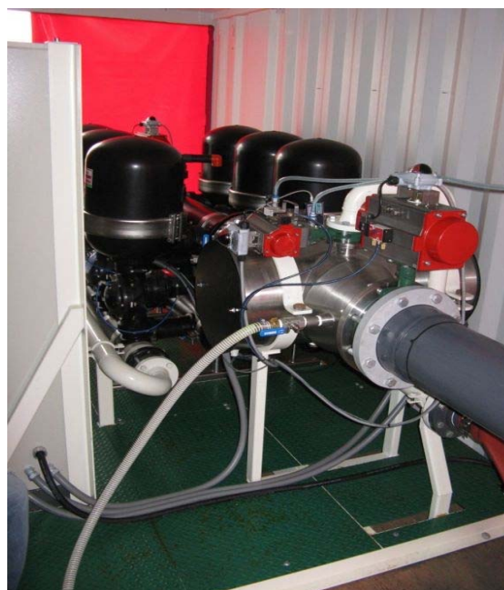
Figure 7. Hyde Guardian containerized test system at NIOZ.
