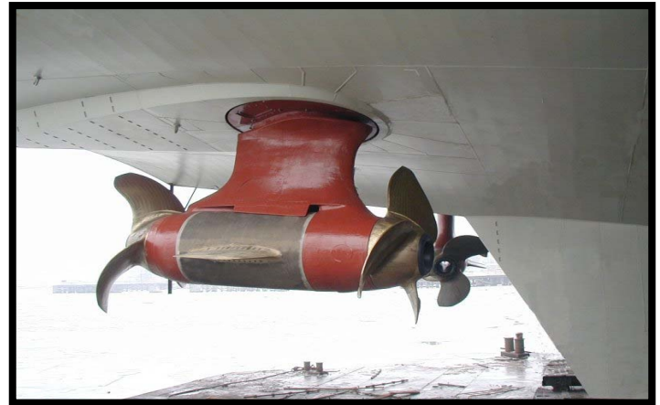
Figure 10: 2000kW Pod Drive Type SEP 2
