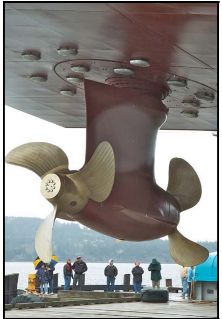
Figure 1 Lower part of a twin propeller Combi Drive
