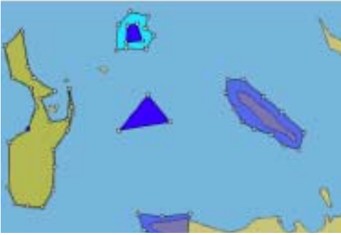
Fig. 8. Defining grounds or depth curves with polygons in the GRISK program.
