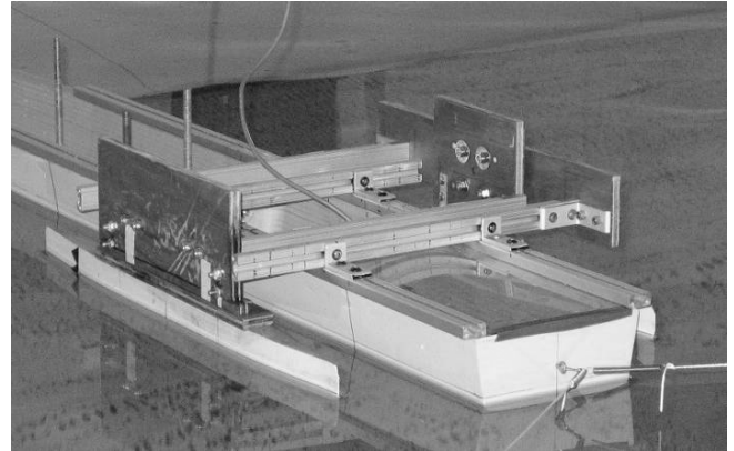
Fig. 1 Photograph of trimaran model with side-hull apparatus
