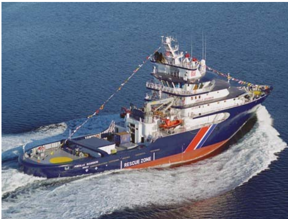
Figure 9 – UT 515 CPV for France combines very high bollard-pull with a high ship speed.
