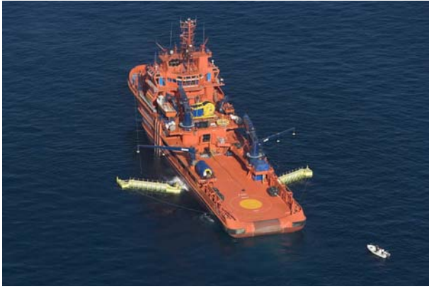
Figure 8 – UT 722L Emergency towing and pollution control vessel for Spain showing oil booms extended.
