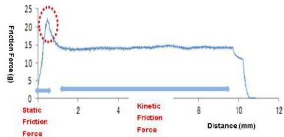
**Figure. 5: The highest friction force is generated just before sliding begins (3)**
