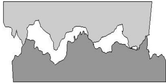
**Figure. 4: Asperity interlocking (3)**
