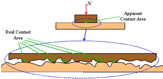
**Figure. 2: Asperities, Valleys, Real, and Apparent contact areas (2)**
