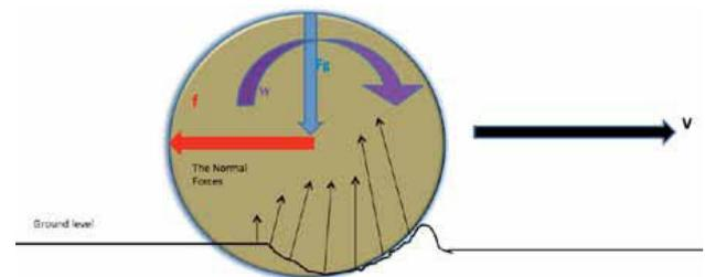
**Figure. 8: Surface deformation at point or line of contact and load transfer (3)**
