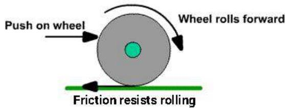
**Figure. 6: Rolling friction**
