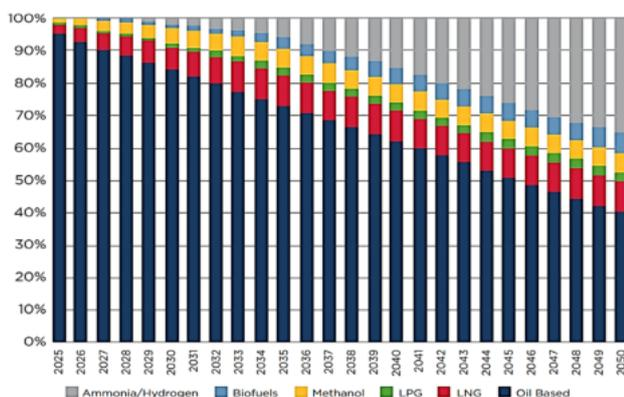
**Figure 7 Prognosis of marine fuel use (Source: ABS 2020)**
