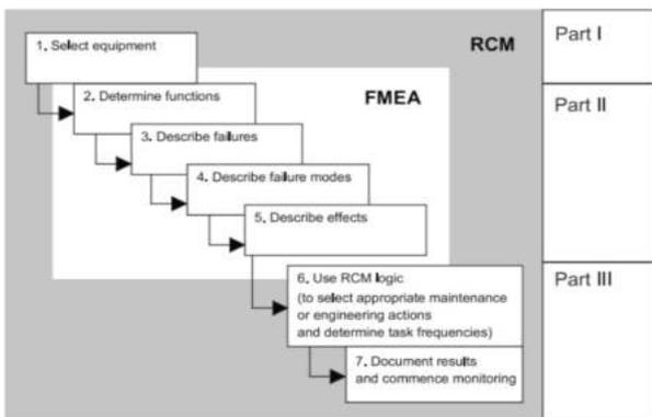
Figure 1: Failure mode and effects analysis [12]
