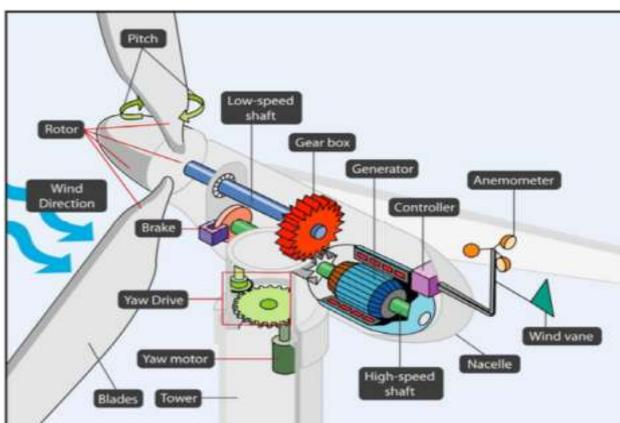
Figure 2: Wind turbine component [13]
