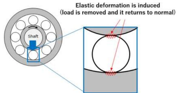
**Figure. 9: Elastic deformation in the area of load (4)**
