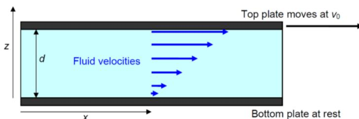
**Figure. 11: Fluid velocity under shear for Laminar Flow (6)**
