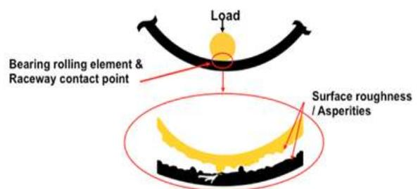
**Figure. 10: Friction due to surface roughness (5)**
