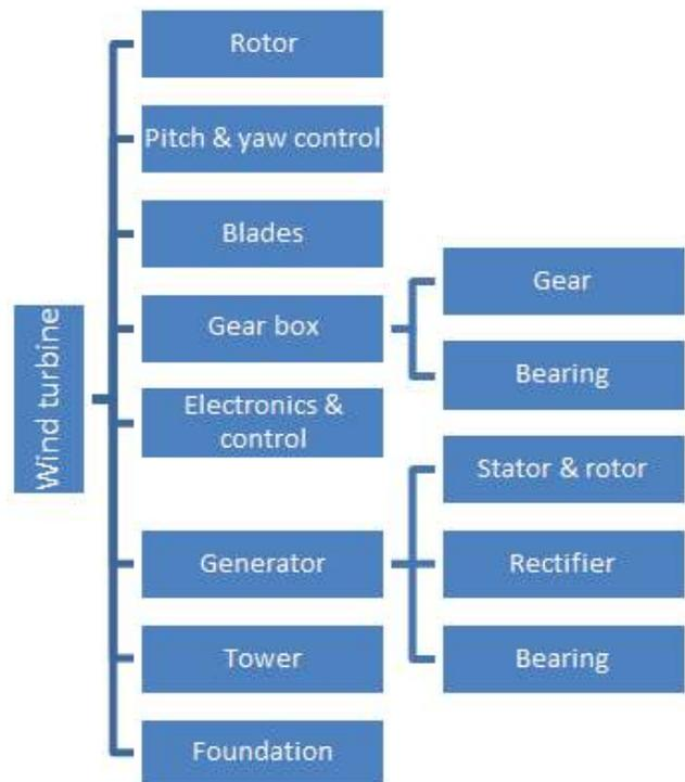
Figure 3: Wind turbine sub structure decomposition[4]
