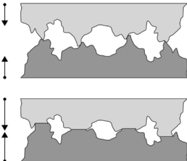
**Figure. 3: (Top) Asperities under no load; (Bottom) asperities under load (6)**
