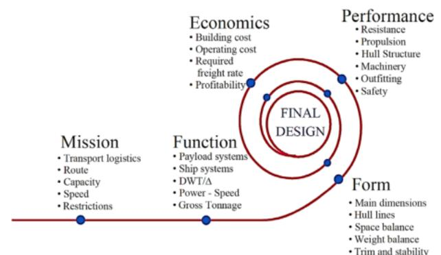
**Figure 8 Ship Design Process (Source: Papanikolaou A., 2014)**
