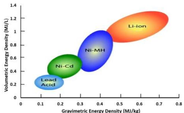
**Figure 11 Energy Density of Batteries (Source: NASA)**
