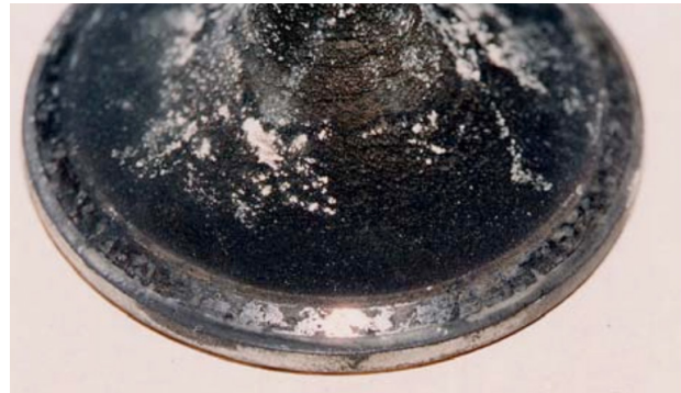
Figure 7. Hard glazed deposits on valve (5)
