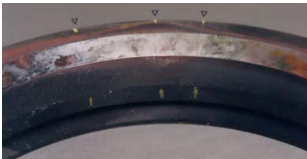
Figure. 10. Exhaust gas blow by through cracked seat (5)
